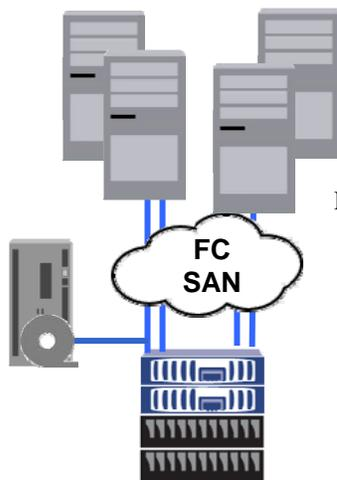
In the SAN-based server-free backup and restore model, data is transferred directly between storage devices (for example, from disk to tape) without using host servers. The server-free backup and restore model significantly reduces application host CPU cycles, thereby freeing up valuable CPU cycles to improve operating efficiency and enable higher workloads across the enterprise.
