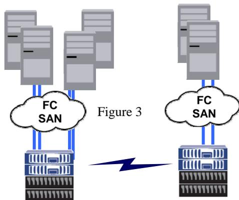
Data access over long distances is a key component of any business continuity solution. Native Fibre Channel technology provides extended distance connectivity of up to 120 km. This distance enables enterprise customers to maintain geographically separate disaster recovery facilities or mirroring operations. When used in large fabric configurations, SANs can utilize Wide Area Networks (WANs) or Metropolitan Area Networks (MANs) to cover even longer distances.
